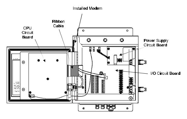
Figure 2-4: LTC-MAP 2130 (Top View with Face Panel Open)
